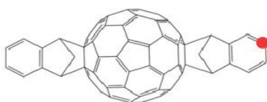
Figure 1. Molecular structure of Indene-C 60 -bisadduct (ICBA)
